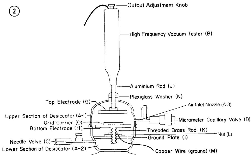
Fig. 2. Drawing of a central vertical section through the glow discharge unit. Same symbols as Figure 1.
