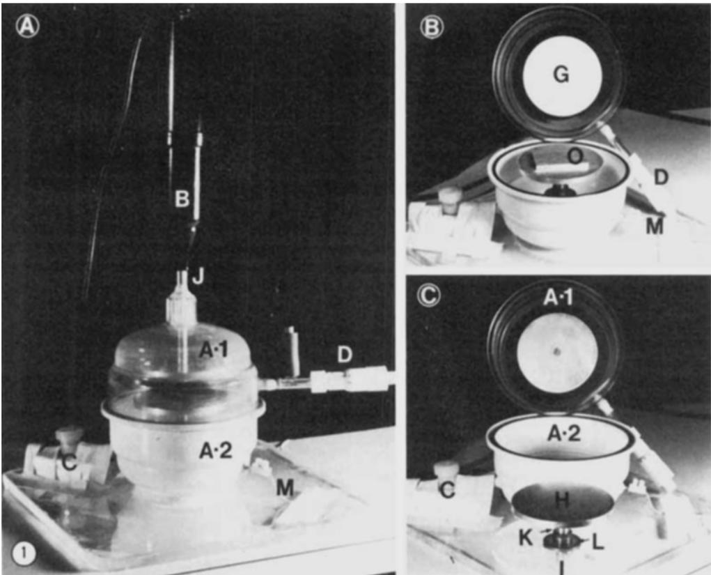
Fig. 1. Photographs of the glow discharge unit; a,b,c show various views. A-1 Upper section of dessiccator; A-2, lower section of dessiccator; B, high-frequency vacuum tester (Tesla coil); C, needle valve connecting chamber to vacuum line; D, micrometric capillary valve; G, upper
